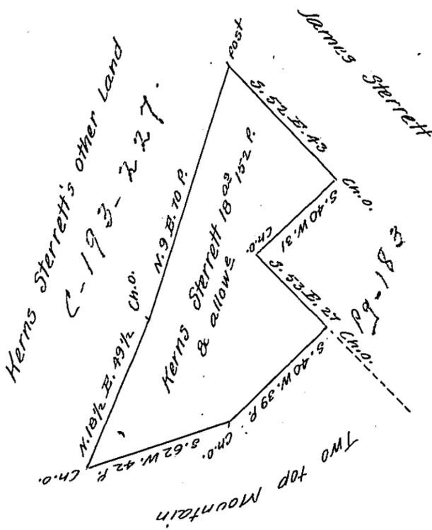
A Draft of a piece of land situate in Montgomery Township in the County of Franklin containing eighteen acres 152 Perches & the allowance of six P. Cent &c. Survey, @ 29<sup>th</sup> May 1794 (under the direction of the late — Math<sup>w</sup> Henderson Esq<sup>r</sup> D. S.) in pursuance of a Warrant granted to Kerns-Sterrett bearing date 24<sup>th</sup> April 1794.
